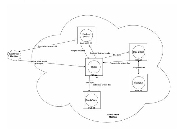
The major change made was modifying the virtual machine structure from including each program in its own virtual machine, to having each program included in one virtual machine.
