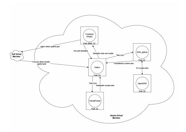
Figure 2: Complete Flowchart of Operation
